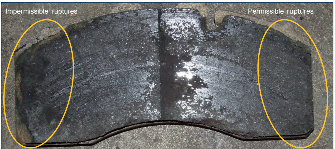
Figure 3: Lining with impermissible
