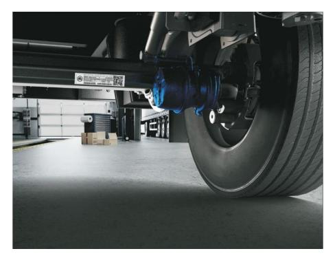
By using a mobile phone or a tablet the workshop can scan the QR code and immediately the user will be directed to the BPW website where one can download the correct spare parts list together with workshop manuals, assembly and operating instructions. The BPW QR code application is intuitively operable and follows the look and feel of online shops.
