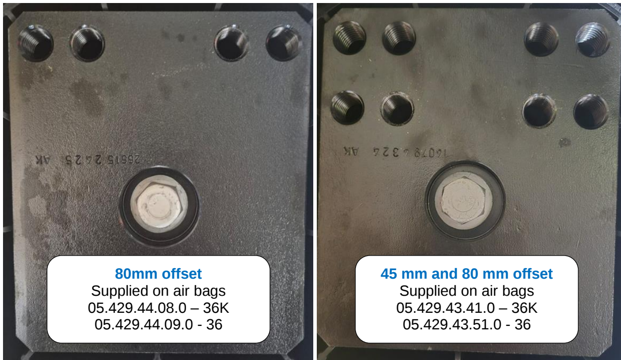
Figure 2: Difference between air bag bottom plates with 80 mm only offset (left) and 45 or 80 mm offset (right)
